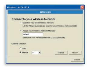
In the Ad-Hoc mode, you can allow the Print Server to automatically associate with another wireless station, or you can manually assign the SSID of your wireless network. You can allow the Print Server to automatically select the channel that is the same as the wireless station with which you want to connect, or you can manually assign a channel.
